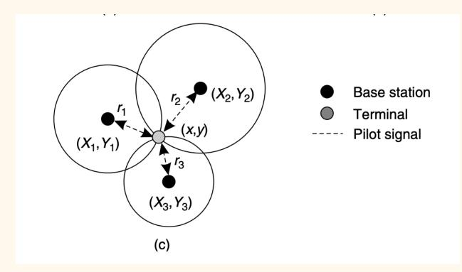
This is called circular lateration in 2D and spherical in 3D. Technically in 3D we need four spheres, not three, because there are two points where three spheres meet, but oftentimes the other point solved for is impossible (it's on the "other side" of the three satellites in GPS, for example!).
