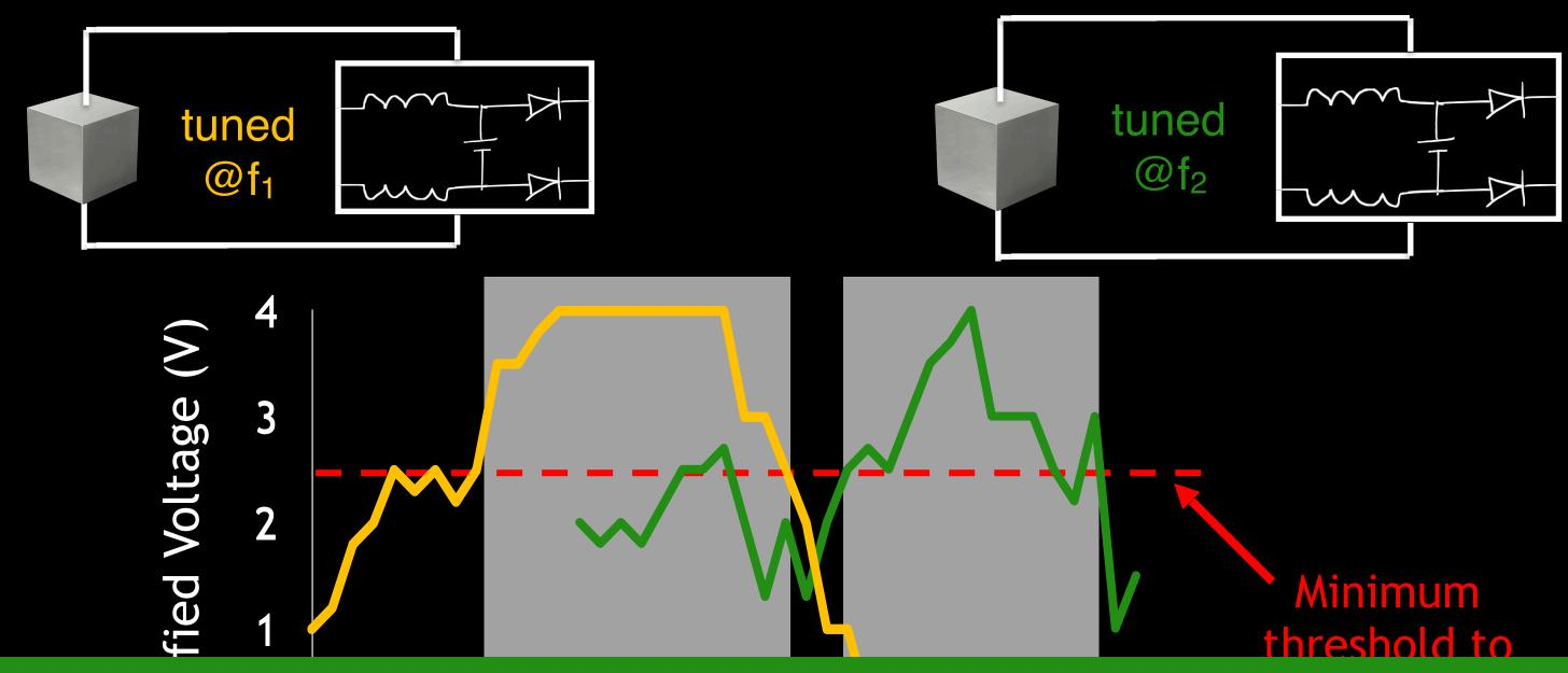
Extend the idea to uplink communication using a MIMO-style decoder adapted to backscatter resonance modes
