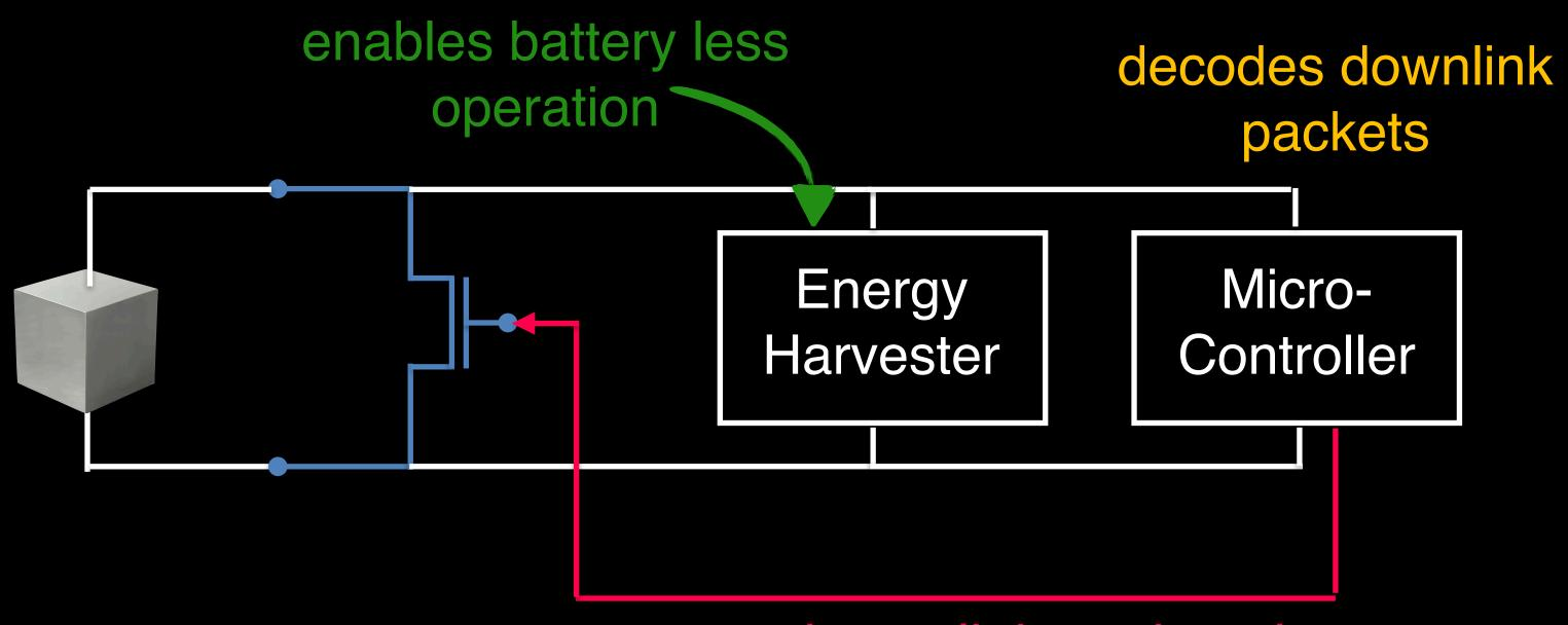
encodes uplink packets by switching transistor
