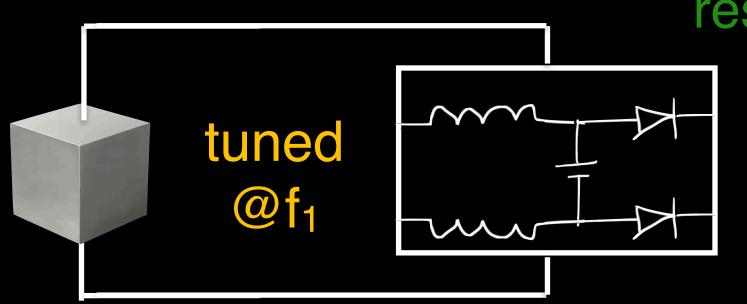
resonance frequency determined by interaction between piezo & the batteryless circuit
