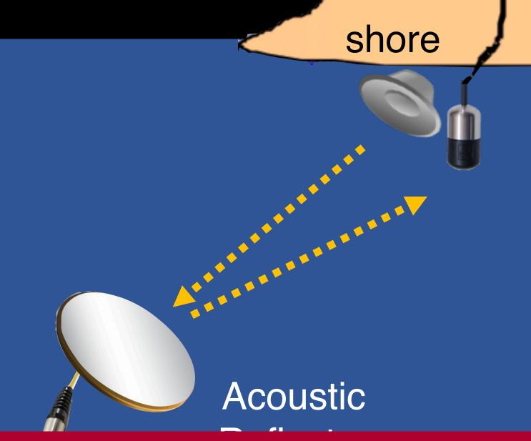
Sensor reflects an existing acoustic signal
