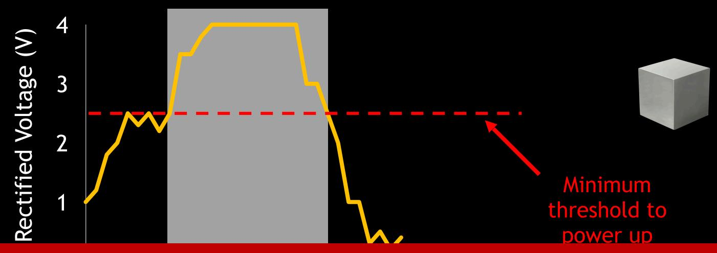
Operating at resonance maximizes energy harvesting but limits concurrent transmissions (and FDMA)
