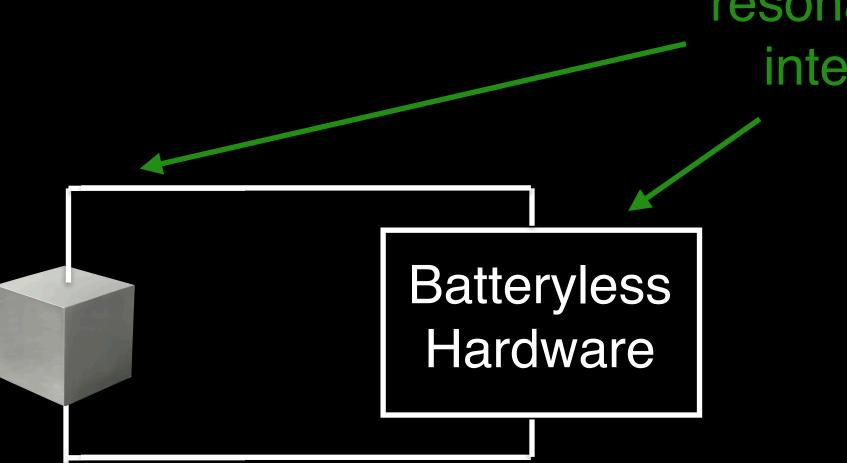
resonance frequency determined by interaction between piezo & the batteryless circuit
