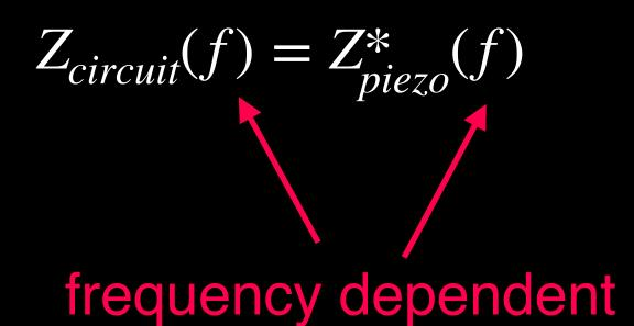
→ Tune the circuit to a different frequency
